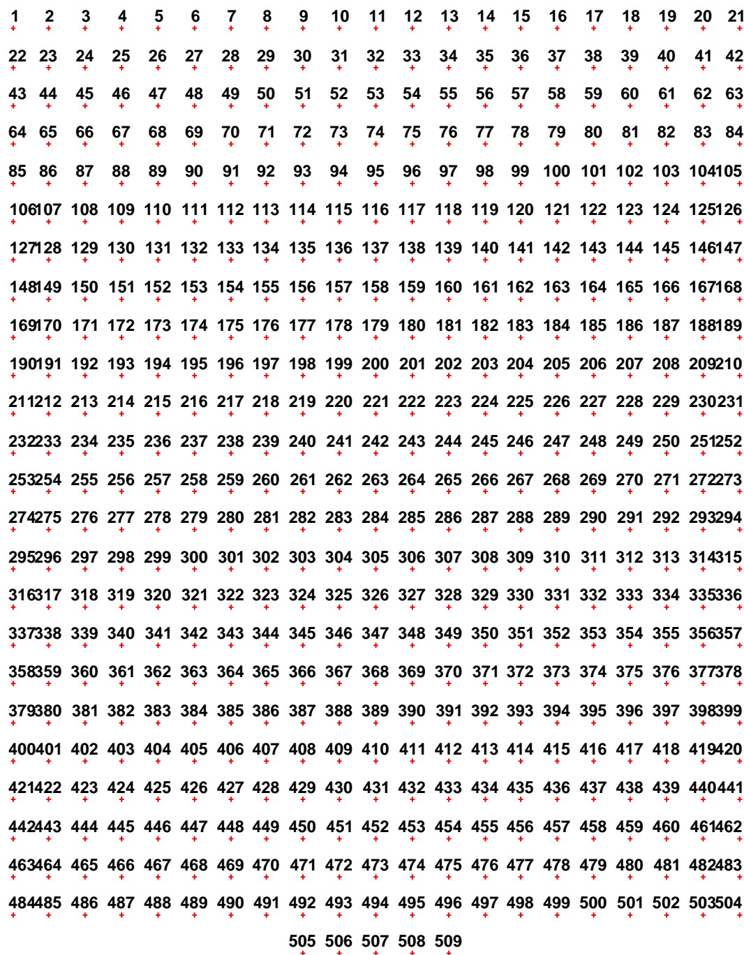
FIGURE 6.30: Electrode layout configuration for material parameter optimisation problem, with 1.6 mm spacing between each electrode in both the x and y directions.
