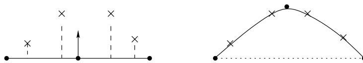
Figure 3.1: Adjusting the nodal parameters of the mesh to minimise the least-squares distance between each data point ( \times ) and its orthogonal projection on the surface. Shown is the effect of adjusting the nodal and derivative parameters of the middle node and the derivative values of the end nodes.
