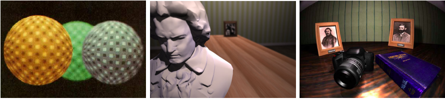
Fig. 6. Images synthesized using distributed ray tracing using a thin lens model (left), thick lens model (center), and a full lens system (right). The full lens simulation exhibits noticeable barrel distortion. (Left image courtesy of Robert L. Cook [5]. Center and right images courtesy of Craig E. Kolb [10]. All images © 1995 ACM, Inc. Reprinted by permission.)
