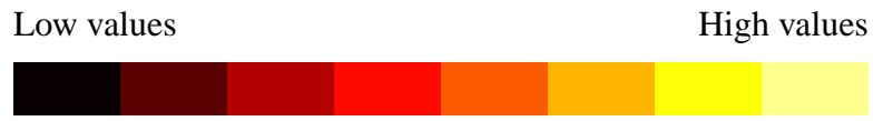
Figure 8.1: Our quantized 8-level “hot” colormap: black \rightarrow red \rightarrow yellow \rightarrow off-white.
