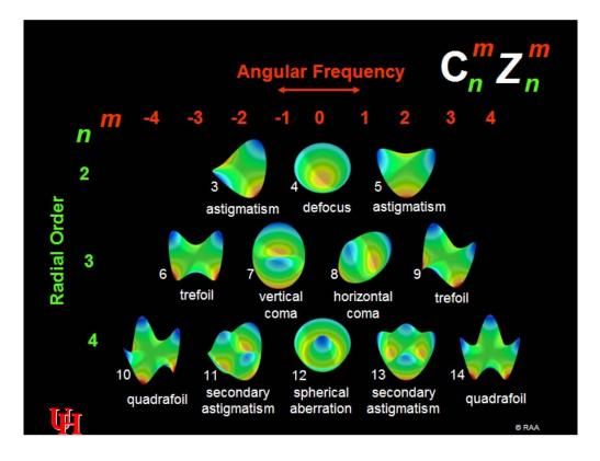
This is your road map to the Zernike expansion. Using the Zernike expansion to represent the wavefront error of the eye parcels the eye's wavefront error into unique building blocks that we can talk about.
