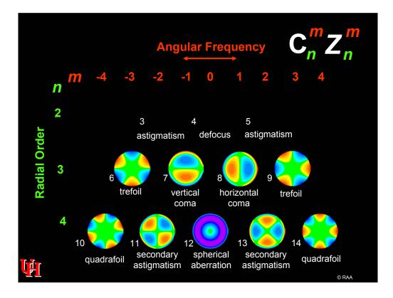
Notice that the WFE is 0 along the horizontal meridian for all radial orders driven by the sin  $\theta$  (i.e., all angular frequencies with a minus designation). This is because when  $\theta$  is 0° it does not mater how many times you multiply  $\theta$ , it will always be 0 (i.e.,  $2 \times 0^\circ = 0^\circ$ ,  $3 \times 0^\circ = 0^\circ$ ,  $4 \times 0^\circ = 0^\circ$ , etc.) and the sin of (0°) =0.
