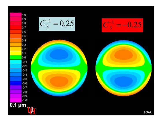
Now let's explore what happens when the sign of the coefficient changes from positive to negative by looking at vertical coma and changing the sign of the coefficient.
