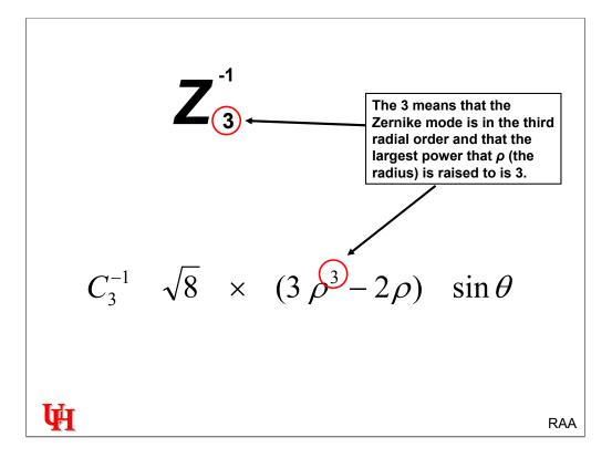
Back to the equation. The subscript designates the radial order and is the largest power that  $\rho$  (the radius) is raised to in the radial polynomial.
