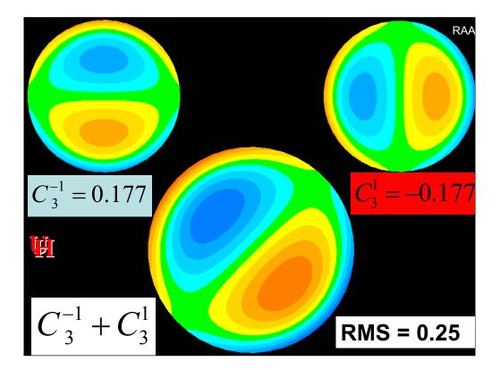
The two coma terms can be added to obtain coma at any orientation. Here I have added equal portions of horizontal and vertical coma but of opposite sign. The result is coma with its orientation in the pupil rotated.
