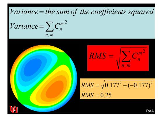
Because we have normalized the coefficients the variance is easily calculated. It is simply the sum of the coefficients squared.
