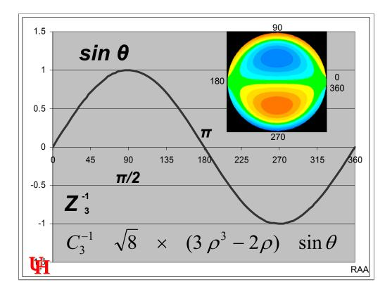
Notice that the sine of theta  $(1 \times \text{theta})$  has a positive portion between 0 and 180 and a negative portion as the angle theta varies between 180 and 360 degree.
