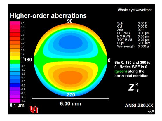
Advanced wavefront errors (i.e., wavefront errors that are in front of the reference wavefront) are warmer colors and have positive values. Retarded wavefront errors (i.e., wavefront errors that are behind the reference wavefront) are cooler colors and have negative values. Green represents 0 WFE. NOTE: This color scheme is currently being debated by the ANSI standards committee. A final answer will hopefully occur sometime in 2003.
