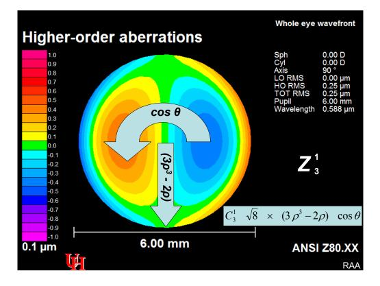
Here we see the horizontal coma mode. Notice that the superscript is now a positive number meaning that angular frequency of the wavefront error varies with the cosine of  $\theta$ . As a consequence the location of the advanced wavefront error (warmer colors) and retarded wavefront errors (cooler colors) have changed location within the pupil. This change in location is being dictated by  $\cos \theta$ .
