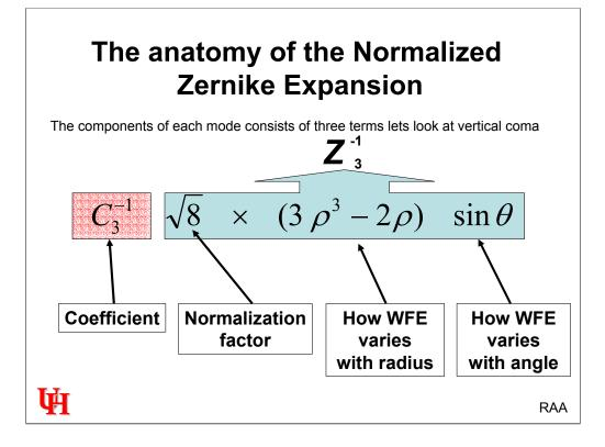
The entire equation for how vertical coma varies within the unit pupil is made up of two major components. The coefficient (shaded in red) and the radial polynomial (shaded in light blue). The same components make up each mode as can be seen in the next slide which details the Zernike expansion for all modes through the 4<sup>th</sup> radial order.
