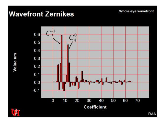
Looking at a graph of coefficient values of the Zernike modes through the 10<sup>th</sup> radial order we see that the two major contributors to the total RMS are term 7 (vertical coma) and term 12 (spherical aberration).
